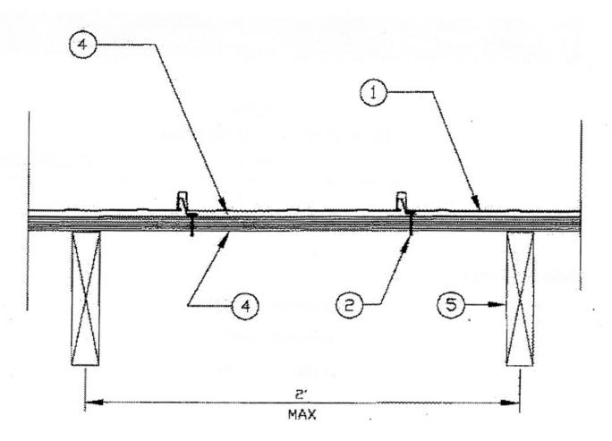
1. Metal Roof Deck Panels\* — No. 29 MSG min coated steel. Max panel width 24 in. Rib height nominal 1 in. Panels continuous over two or more spans. A bead of sealant may be used at panel endlaps.
