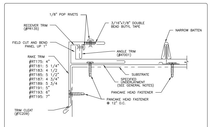
NOTE: FIELD CUT FIRST AND LAST PANELS TO EQUAL WIDTH.
